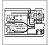
3 Remove the wire contact screws L-N-, then fasten the wires under the screw heads, respecting the colour code: Black/Blue (N), Red/Brown (L) and Bare Wire/ Yellow-Green (\_\_).
